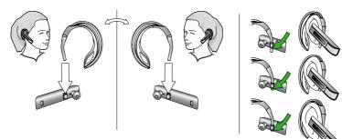
Figure 42: Attaching the ear hook
